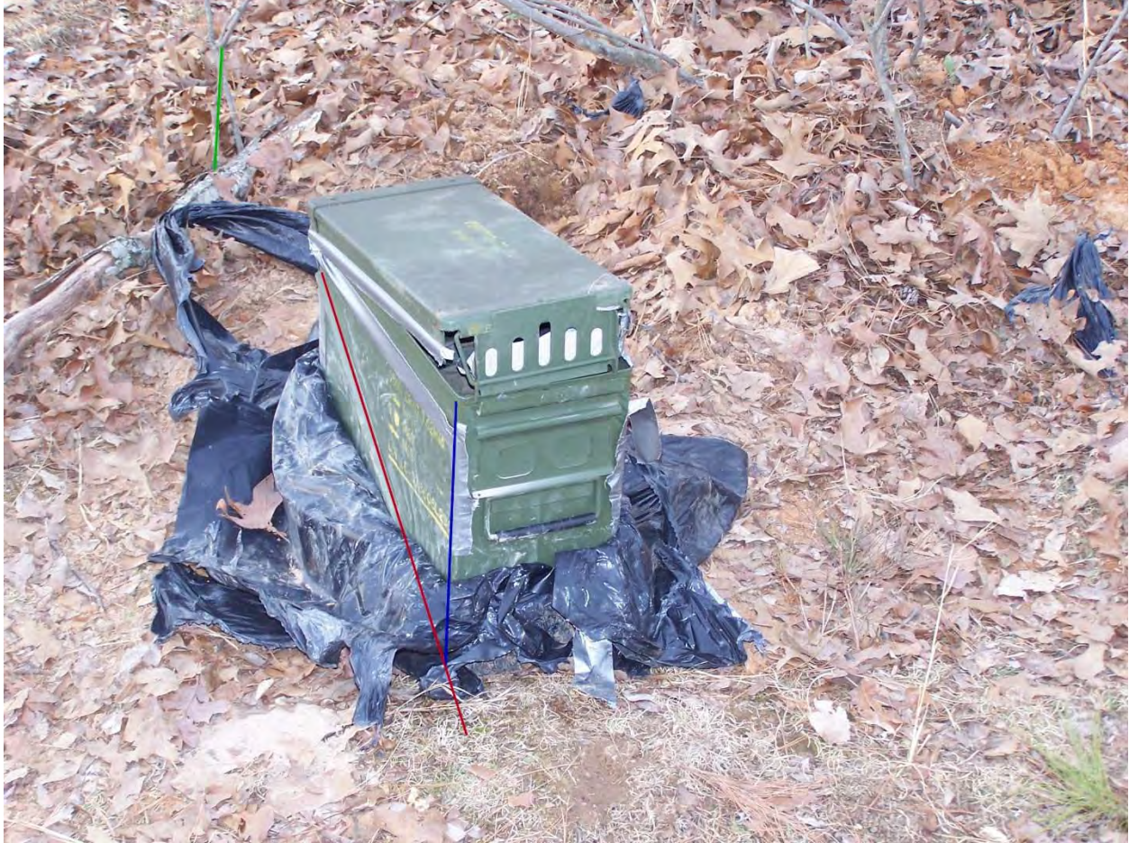
Figure 3-4. Marks on the photograph to enable measurement on the canister and the reference object
