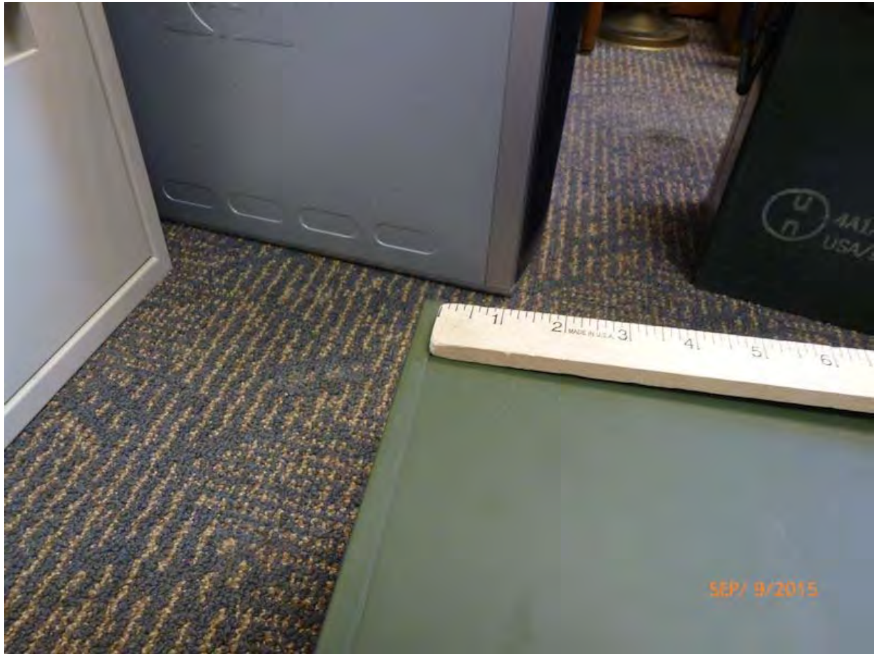
Figure 3-5. Photograph showing the top of the partial height and the bottom of opening ring (the extra metal piece at the opening of the canister)
